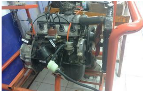
Figure 3.3. Toyota Kijang 4k Series Engine
